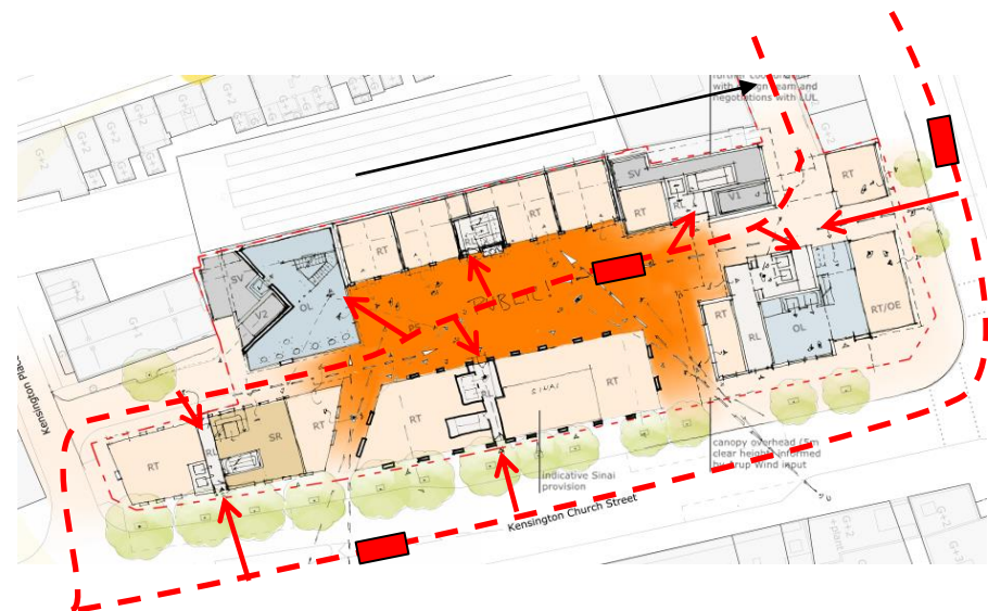
Figure 1. Fire Service vehicle and personnel access routes.
